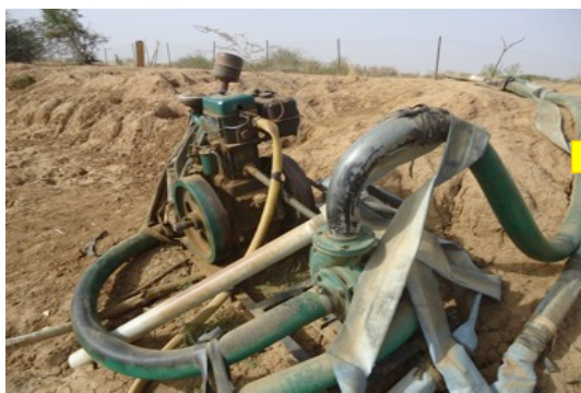
Figure 27: Diesel generator for irrigation water pumping on the AHAs.
